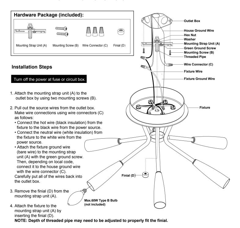
5. Install 6 x 60W Max. candelabra base bulbs (not included). Check relamping label at socket area or packaging for maximum wattage allowed.
